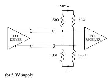
Figure 10. DC-coupling between PECL and PECL
