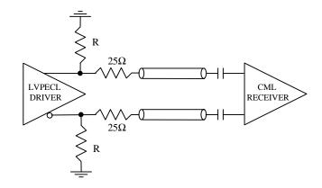
Figure 13. AC-coupling between LVPECL and CML
