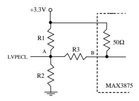
Figure 14. Resistor network between LVPECL and CML (MAX3875)
