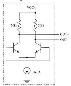
Figure 3. CML output structure
