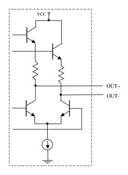
Figure 6. LVDS output structure
