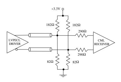
Figure 15. DC-coupling between LVPECL and CML (MAX3875)
