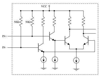
Figure 5. CML input circuit configuration
