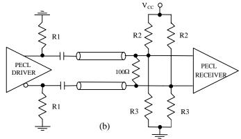
The disadvantage of Figure 11(a) is that the power consumption caused by this termination network is high. For systems where power consumption is a main concern, Figure 11 (b) can be used. In this case
