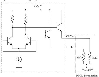
Figure 1. PECL output structure
