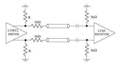
Figure 18. AC-coupling between LVPECL and LVDS
