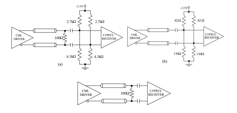
(c) LVPECL with on-chip high-impedance biasing
