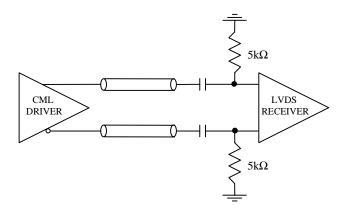
Figure 21. AC-coupling between CML and LVDS
