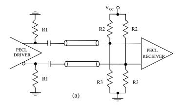
Figure 11. AC-coupling between PECL and PECL
