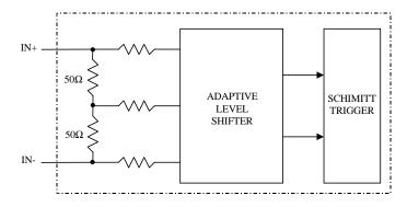
Figure 7. LVDS input structure
