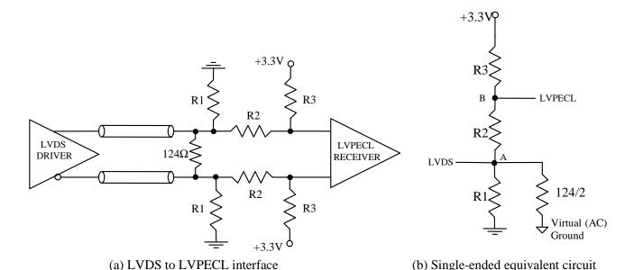
Figure 19. DC-coupling between LVDS and LVPECL
